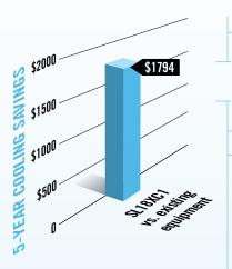
SEER stands for "Seasonal Energy Efficiency Ratio" and is a measure of the cooling efficiency of air conditioners. The higher the SEER, the greater your energy savings. Typical SEER ratings start at 13.00, but the SL18XC1 carries ratings as high as 18.50.
